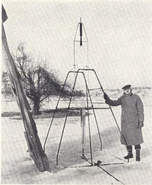
1. Liquid oxygen-gasoline rocket in the frame from which it was fired on March 16, 1926, in Auburn, Mass.
