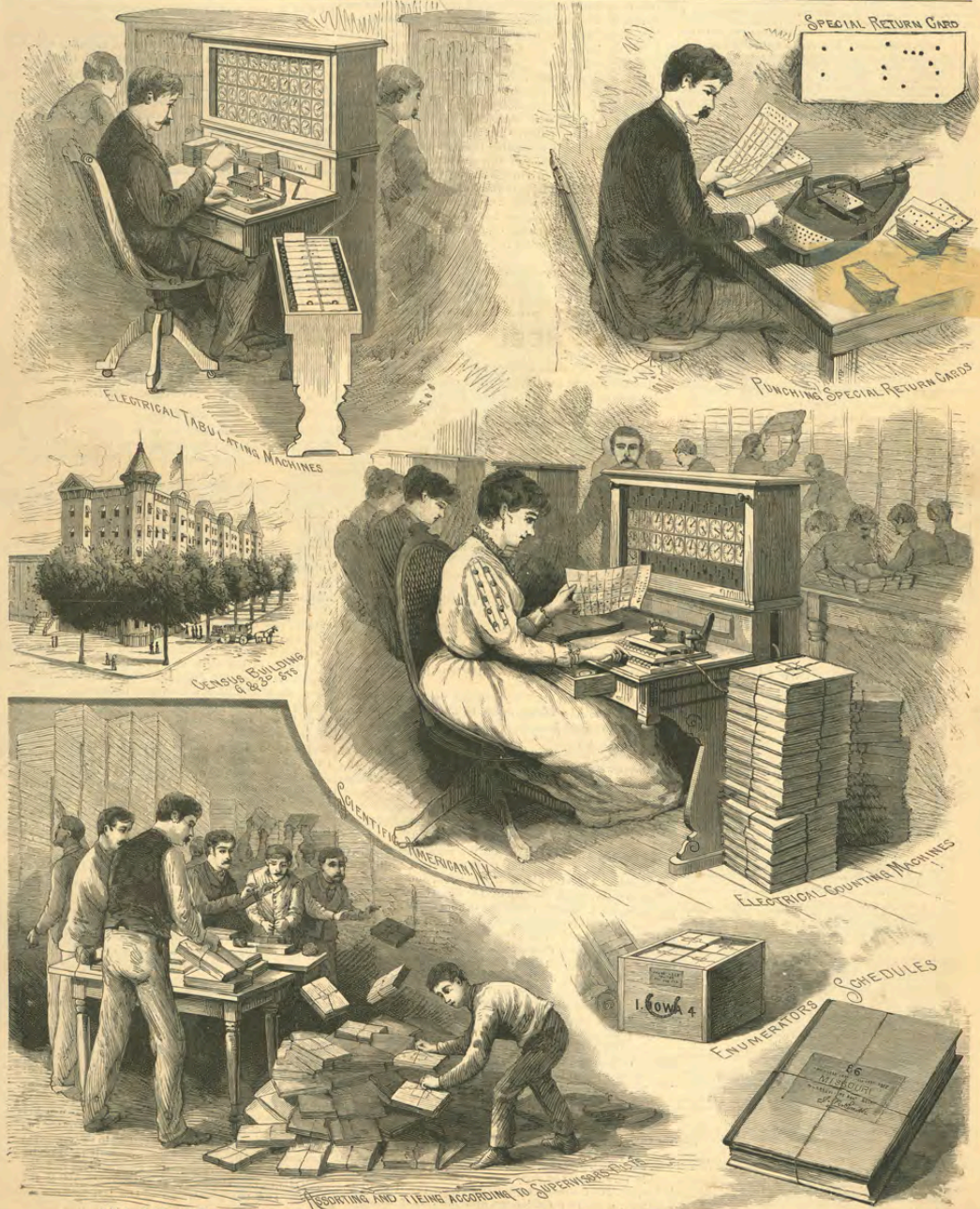
THE NEW CENSUS OF THE UNITED STATES—THE ELECTRICAL ENUMERATING MECHANISM.—[See page 132.]
